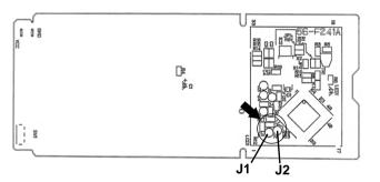
**NOTE** : For modification, take out the batteries and press the OPERATE/STOP (ON/OFF) button twice or 3 times at first. After finish modification, put back the batteries then press the RESET button.
